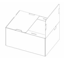
**Step7.** Push down flaps and locking tabs into locking slots to close the box.
