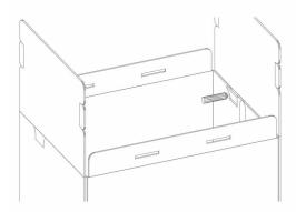
**Step1.** Push the middle of snap fit pins back, bending thru the slots. Or simply pull away side panel to disengage the snap fit.
