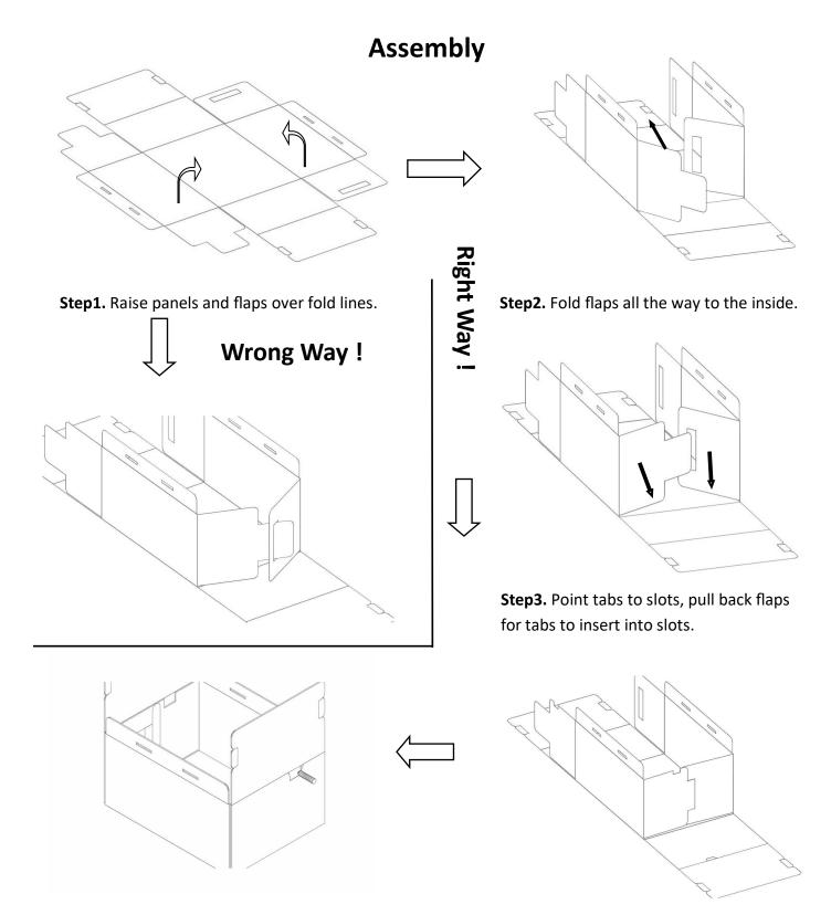
Step5. Raise side panel. Hold flap to panel tight together near snap fit pin. Use finger or pen to push snap fit pin middle, bending thru the slot.
