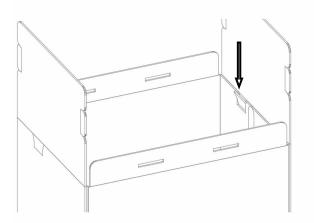
**Step6.** Snap fit pin all the way inside, lock against the slot vertical sides.
